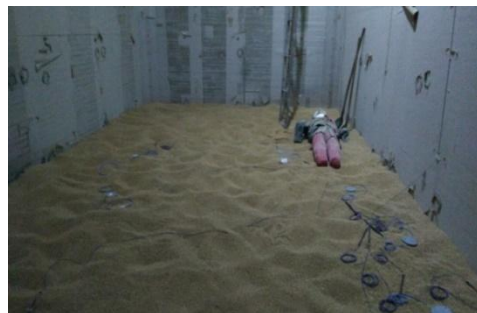
粮库进出粮作业事故模拟试验研究 Study on accident simulation test of filling and emptying operation in grain depots
