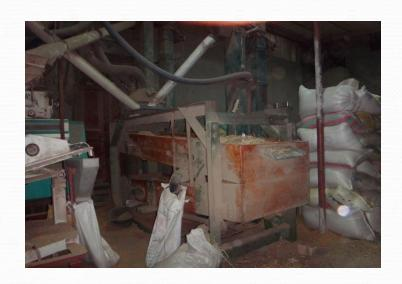
Negative effect for stoneremoving, low output, high broken rice and low efficiency to use the primitive tools
