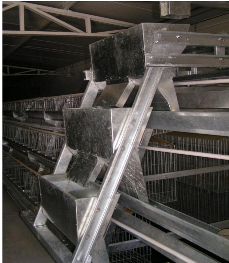
Figure 2-33 Feeding machine in the house
